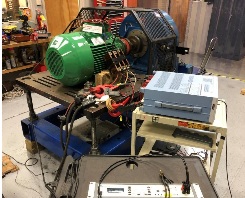
Figure 2: 45HP, 4 pole test setup
