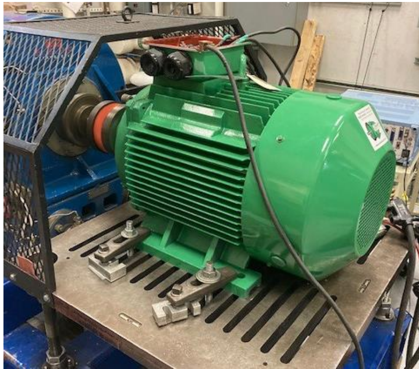
Figure 3: 45HP, 6 pole test setup
