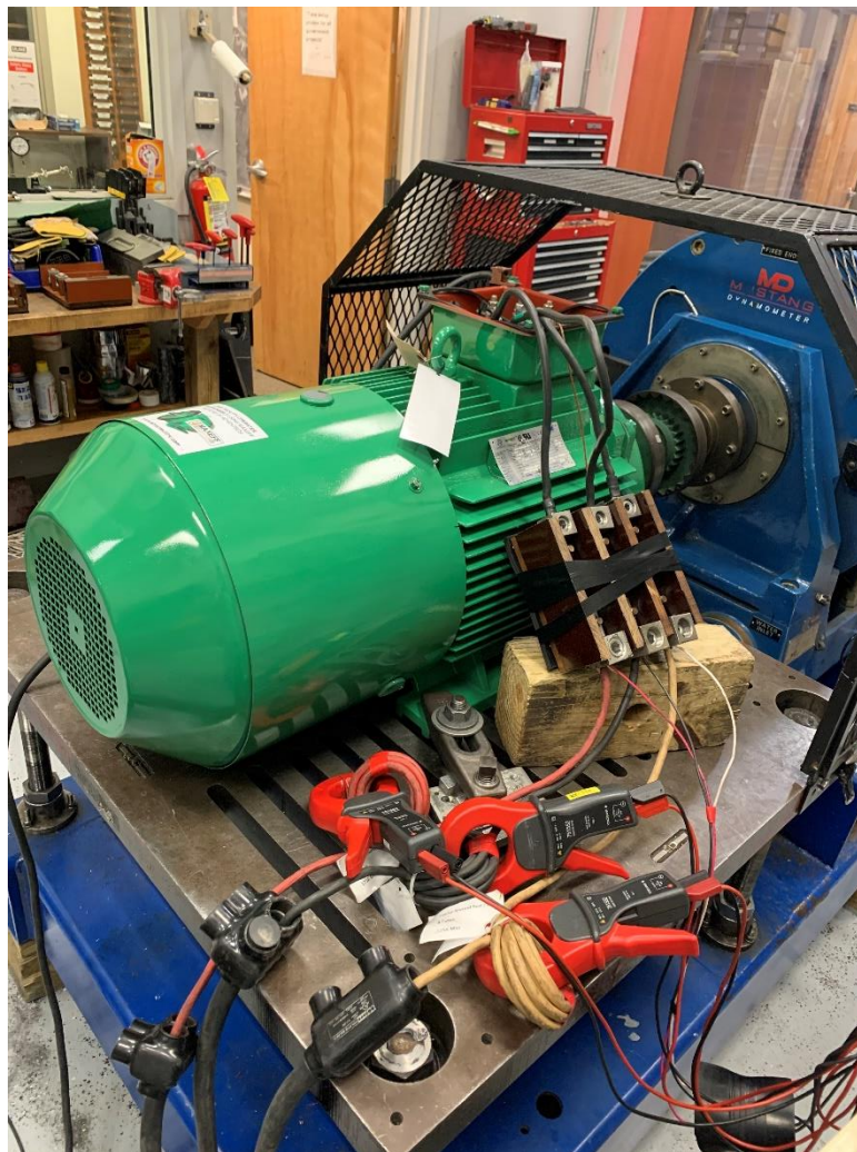
Figure 1: 40HP, 2 pole motor test setup
